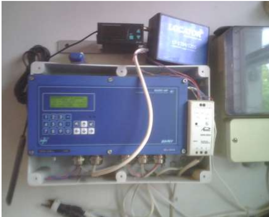
Flowmeter Transducer with Locator Datalogger
